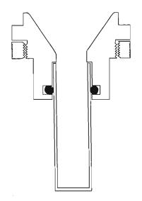
The actual size of the etherizer shown in scale drawing is 50 mm. in widest diameter. A polyethylene tube, with holes that have been poked with a hot needle, is inserted into a hard aluminum alloy head, as shown, with an 0 ring seal at the junction. The etherizer can be
